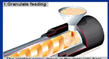
The rotating screw draws in the granulate from the material hopper and transports it in the direction of the screw tip.
