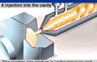
The plastics-gas mixture is under pressure and is injected into the injection moulding tool, where it forms small, finely distributed gas bubbles. Micrograph showing average cell size of 10 microns (.0004 Inches)
