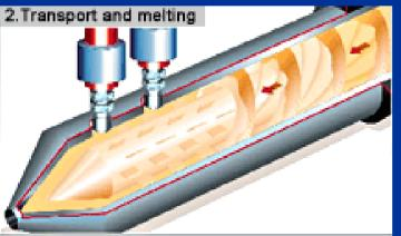
The plastic is platified and homogenized by heating while being transported.
